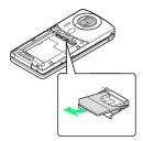
· Lift and slide out USIM Card as shown.
