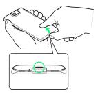
· Use notch  $(\bigcirc)$  to lift Battery Cover.
