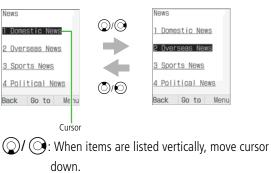
When the page is already scrolled to the bottom, alternatively, press Side Key 🕘 to move cursor down.
