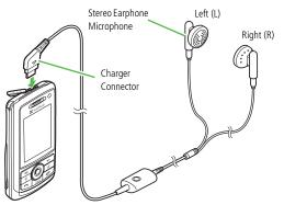
Use Stereo Earphone Microphone to accept Voice Calls. When 805SC rings/vibrates, press Stereo Earphone Microphone switch for 1+ seconds to answer the call.
