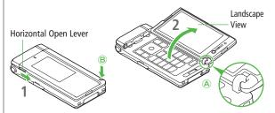
Do not lift hinge portion (B) when opening handset.
